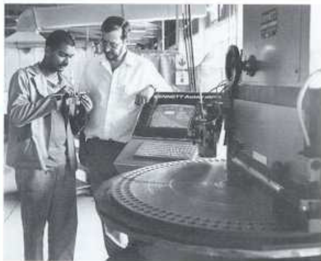
Setter Nireesh Ramjewan and marketing director Buzz Kopp examine a product coming off Webroy's new state-of-the-art CNC spring grinder.
